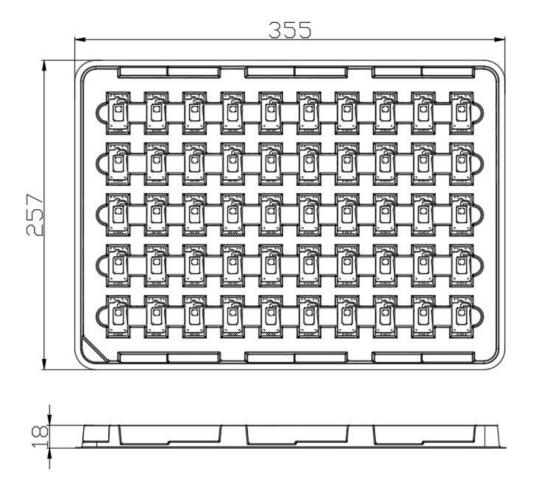
Figure 5. Size of plastic tray (unit: mm)
