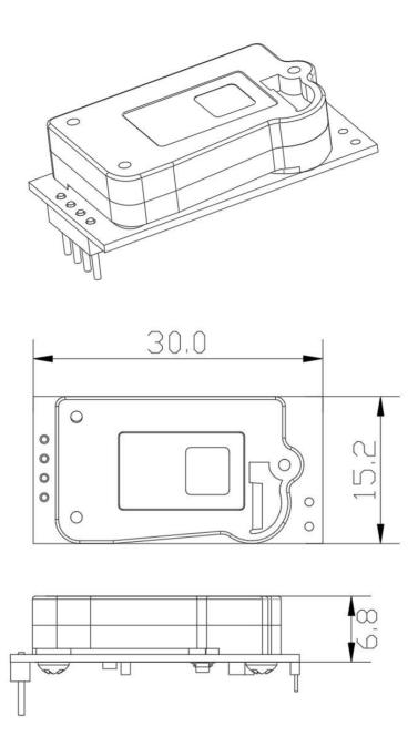
Figure 4. ACD10 dimension (unit: mm)
