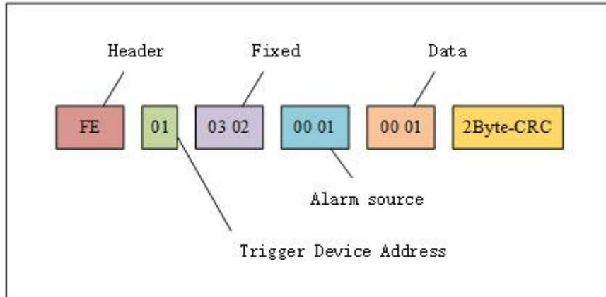
"Header": the first byte, used to identify the data frame as alarm data;
