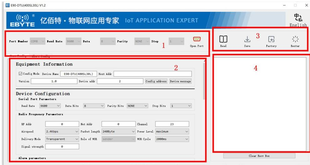
①Area 1 is the parameter configuration area used to connect the radio station, which needs to be configured corresponding to the radio station. For example, if the radio station is configured as 9600-8N1, then you need to select the port number of the USB to serial port connecting the radio station, configure the baud rate to 9600, and the data bit is 8, the parity bit is NONE, and the stop bit is 1;
