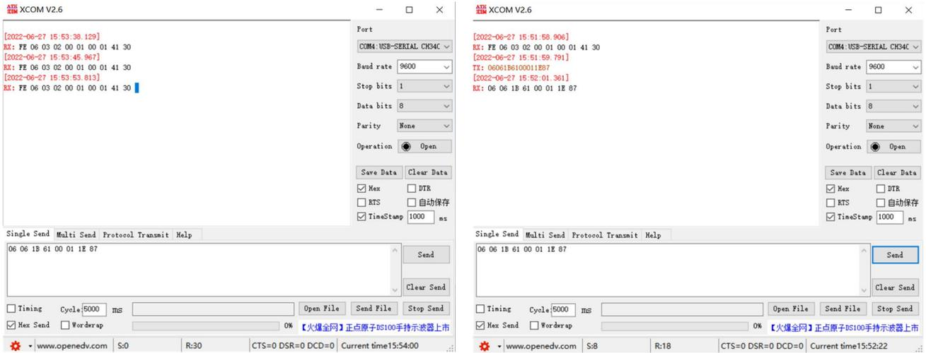
The picture on the left shows the alarm report of the device without clearing after the alarm is generated, and the picture on the right shows the report of the device alarm after manual clearing.
