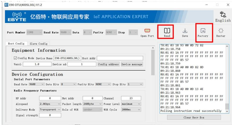
Click "Read Parameters" to know that the default Modbus address of the device is 1. If the serial bus connected to the device already has address 1, the address can be configured to other values here. If Modbus RTU protocol transmission and remote configuration are not performed, it can be ignored. address parameter;
