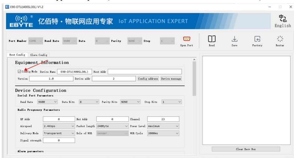
If you remember the device address, you can also modify the device parameters without entering the "configuration mode". For example, the host Modbus address is 1, and the slave Modbus address is 2. You can connect the host radio through the serial port to configure the parameters of the remote slave and local host.
