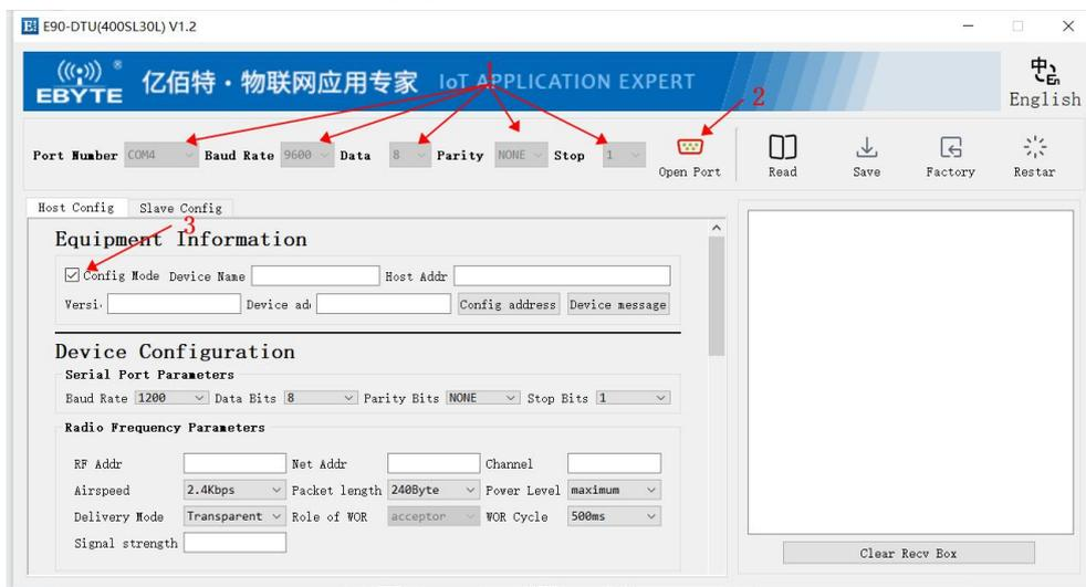
The purpose of the "Quick Start" here is to use the device quickly, and the parameters use the factory parameters. If the device has been configured before, click "Factory Settings" to restore the factory parameters:
