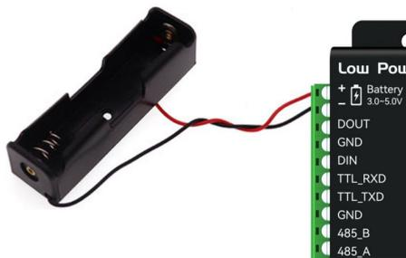
Signal line access, RS-485 or TTL-3.3V, serial ports cannot be used at the same time, only one of them can be used at the same time:
