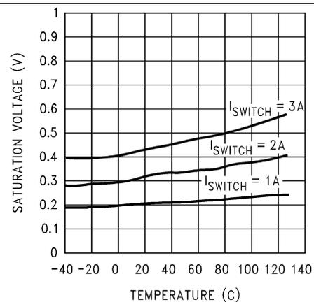
Figure 6. Switch Saturation Voltage vs Temperature
