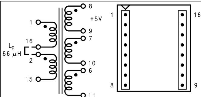
Figure 36. Pulse PE-68413 (Top View) (Surface Mount)
