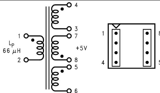
Figure 31. Coilcraft Q4338-B (Top View)
