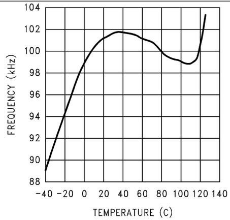
Figure 8. Oscillator Frequency vs Temperature
