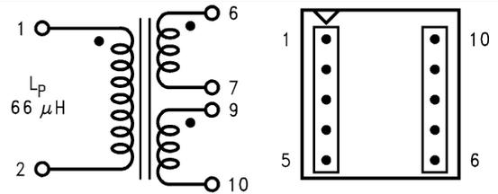
**Figure 41. Schott 67140900 (Top View)**
