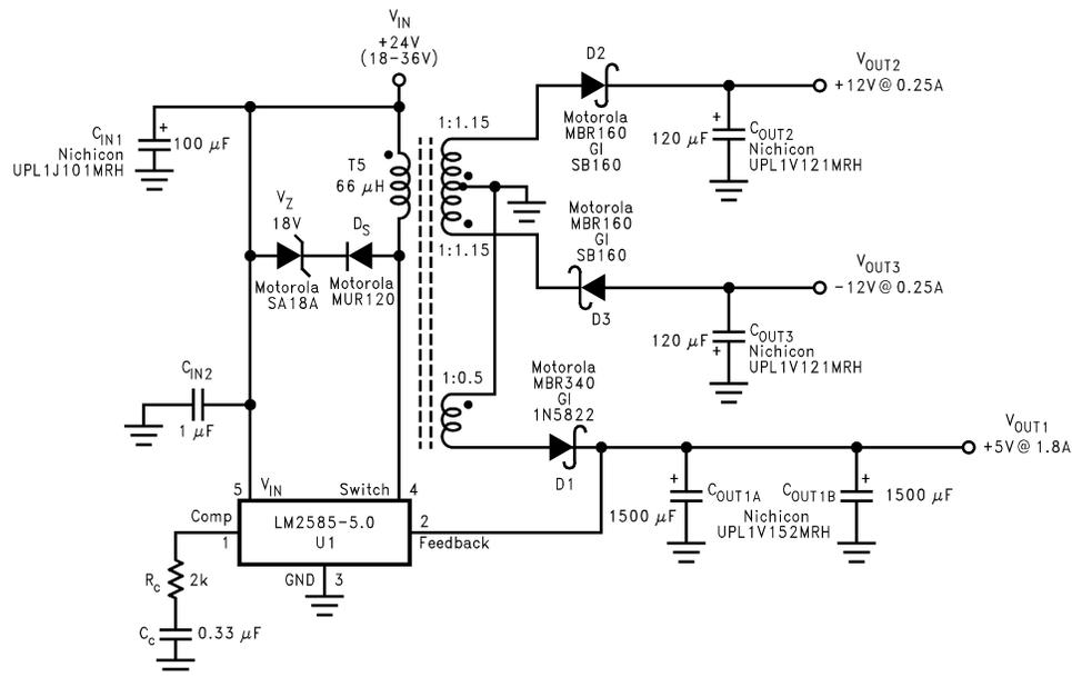
Figure 27. Triple-Output Flyback Regulator
