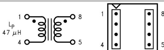
Figure 34. Pulse PE-68482 (Top View)
