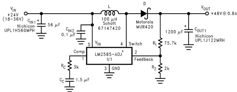
\*The LM2585 will require a heat sink in these applications. The size of the heat sink will depend on the maximum ambient temperature. To calculate the thermal resistance of the IC and the size of the heat sink needed, see [Heat Sink/Thermal Considerations](#)
