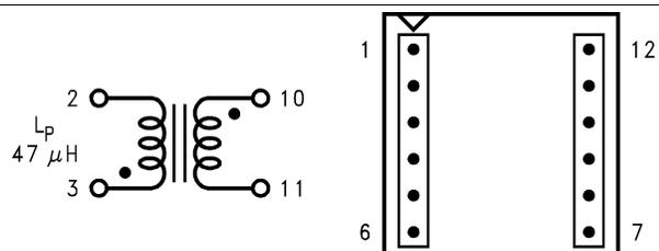
Figure 32. Coilcraft S6057-A (Top View) (Surface Mount)
