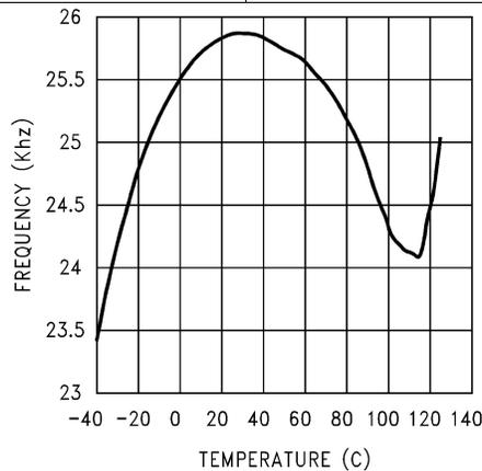
Figure 11. Short Circuit Frequency vs Temperature
