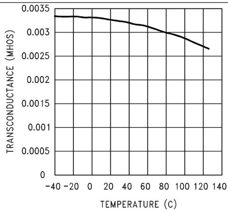
Figure 9. Error Amp Transconductance vs Temperature
