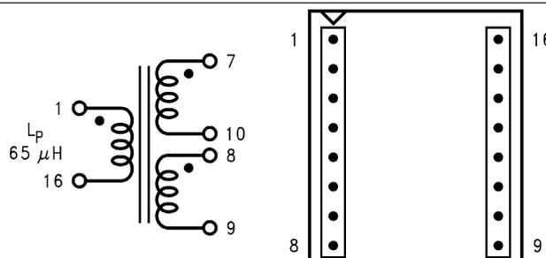
Figure 35. Pulse Pe-68414 (Top View) (Surface Mount)
