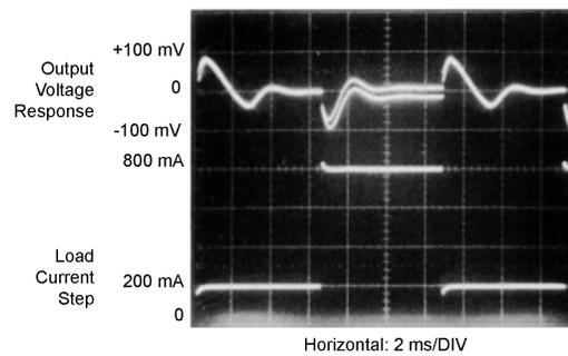
**Figure 17.  $V_{OUT}$  Response To Load Current Step**
