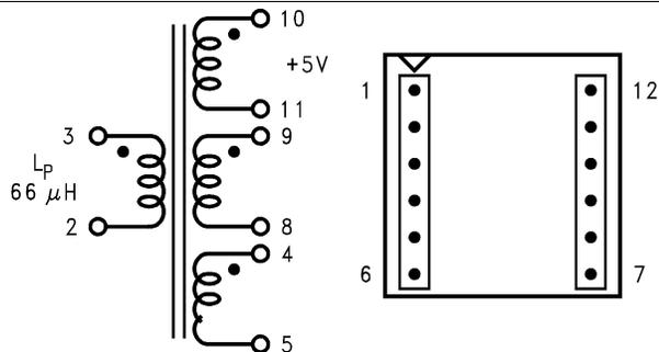
Figure 30. Coilcraft Q4437-B (Top View) (Surface Mount)
