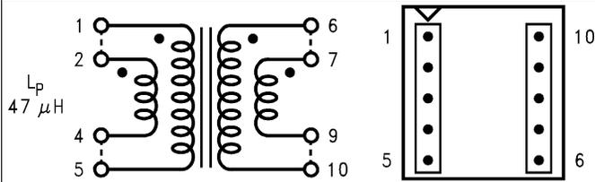
**Figure 40. Schott 26606 (Top View)**
