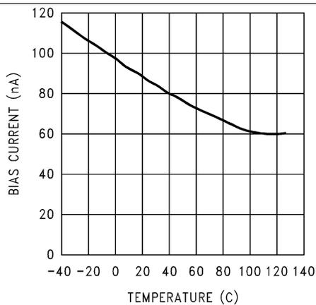
Figure 5. Feedback Pin Bias Current vs Temperature
